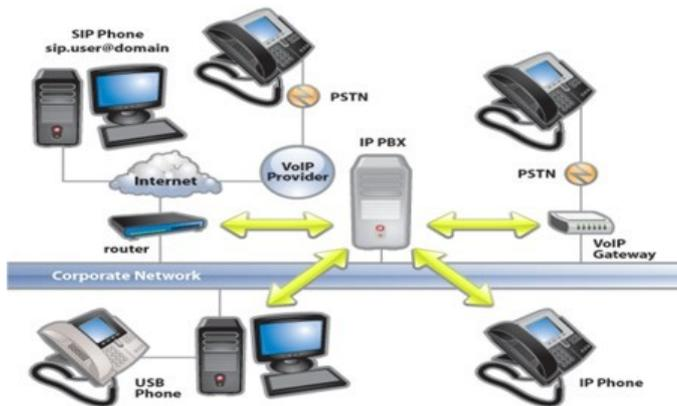
We know that a **PBX System** is a telephone switching system that provides communication between a number of phones and trunk lines for departments within a company.
